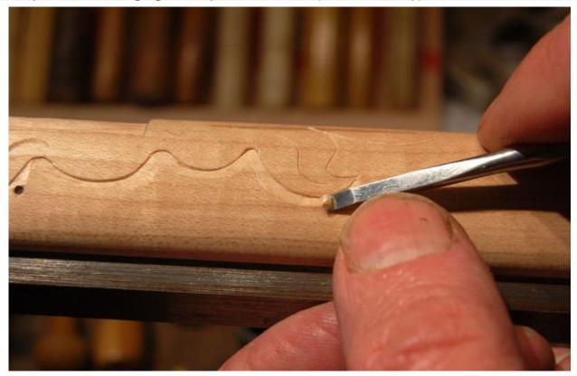
Blend the background down with a flattening rasp. Fair it out as far as practical, and tip the stock in the light to make sure the divots and bumps are all flattened.
