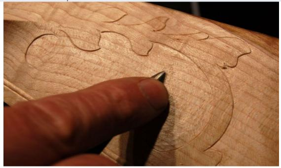
I made this rasp. Takes a couple of hours to do so, but it saves centuries of leveling with a scraper. This tool is very aggressive, with pointy little teeth like a Jack Russel, so take it easy with the pressure. Make the shape you want, then raise little teeth with a graver or small chisel. Then harden. Use spring steel or 0-1. This one is low carbon steel, case hardened. Pain in the butt to go thru that process for one tool.
