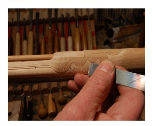
The scraper is very useful for shaping the transitions. Just roll the stock in the light, and you will see where material needs to come off.
