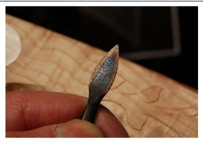
View of scraper I use. 1/32 thick 0-1 tool steel. I hardened it and drew it back to spring temper. Lately I have been simply grinding the end square and sides flat, ie: not rolling a burr.
