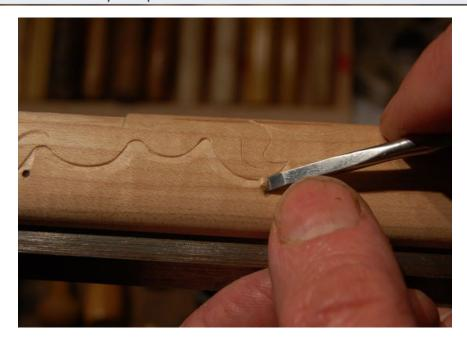
A very sharp scraper makes quick work of leveling and working up to the relief. Note that the relief is very shallow, maybe .02" at most.
