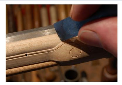
I keep the ramrod in the stock so I don't mess up the knife edge of the RR channel and pipe inlet.
